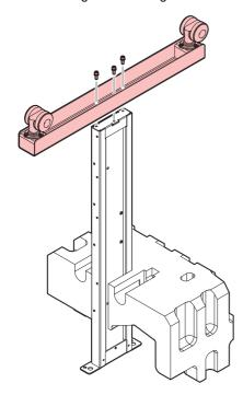
3 Remove the cushioning material and turn the legs back in their original direction.
