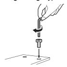
2 Push the hex wrench into the tightening pipe and retighten the screw.
